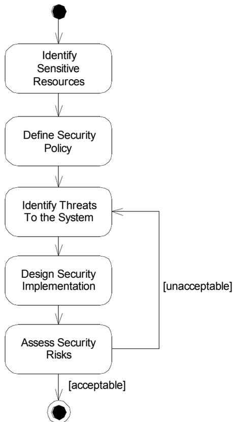
**Figure 1. Security Perspective Process**
